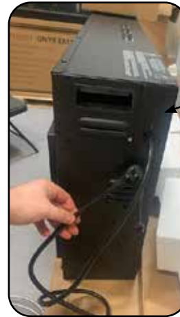
Wire Harness & Cover Plate Reinstalled.
